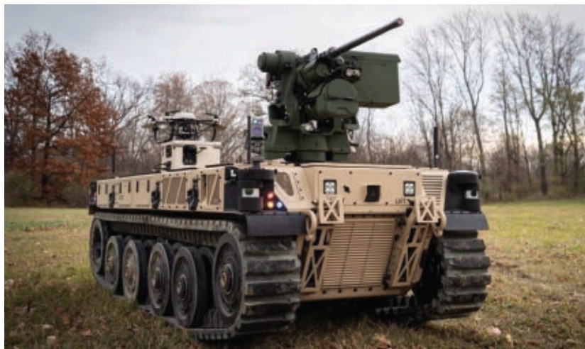
▲ The U.S. Army Ground Vehicle Autonomous Pathways program prototypes software for the navigation of uncrewed vehicles by fusing data from multiple sensors and allowing teleoperations of unmanned ground vehicles. Army photo.
